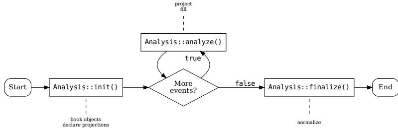
Figure 1: Sketch of the RIVET program flow, with initialization, analysis and finalization steps, as described in the text. Figure from [3].
